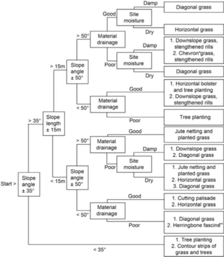
Fig. 2.9. Example on how to standardize decision making for different slope angles, drainage material and moisture conditions. Some plants are Nepal specific, e.g. jute. Therefore, it needs to be adapted to the Kyrgyzstan context. (*Chevron is a zigzag pattern ** Herringbone is a diagonal pattern); Source: Devkota et al, 2014
