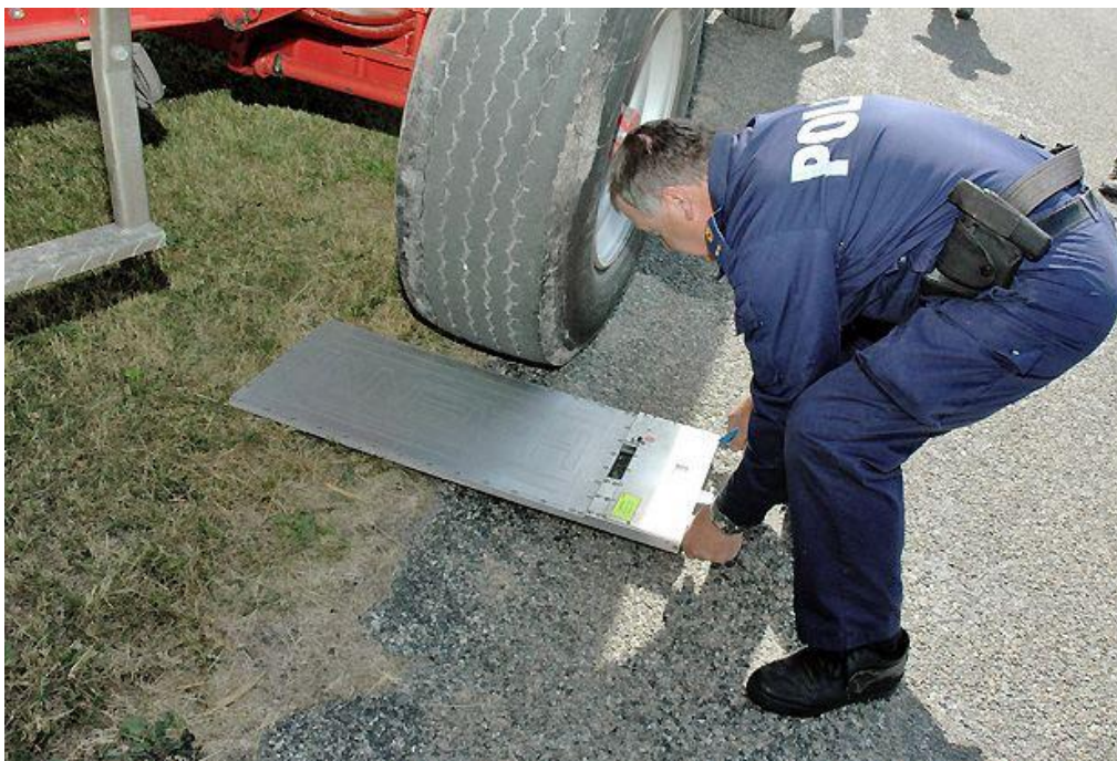
Fig. 2.4b The Police in Switzerland uses mobile scales for control of axle weight. (Source: Schweizer Bauer, Heinz Röthlisberger)
