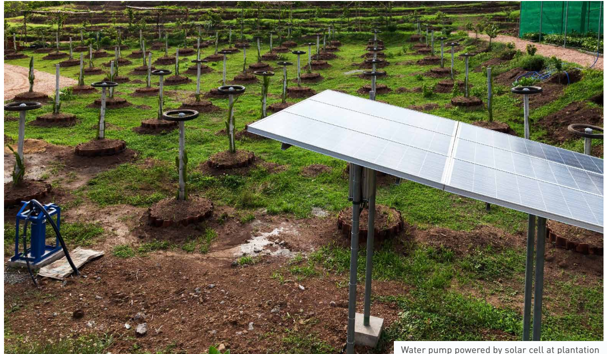
Water pump powered by solar cell at plantation
