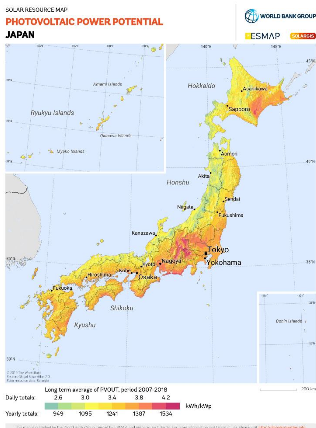
Figure 2: Photovoltaic power potential in Japan considering technical limitations
