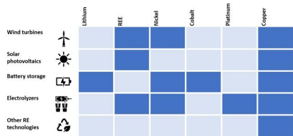
Figure 1: Use of selected CRMs by energy transition technologies covered in this report
